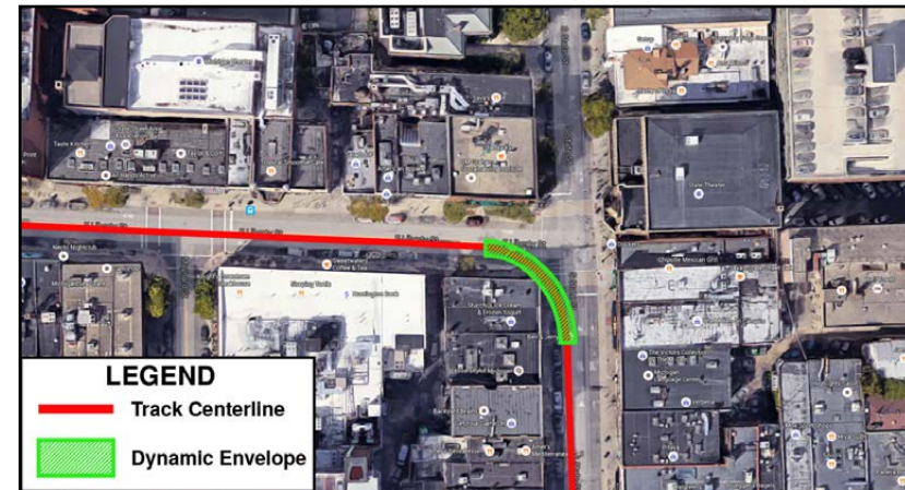
Typical intersection right-of-way concern
