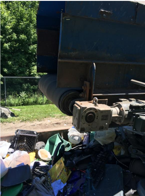
Corrected material build-up on conveyer roller
