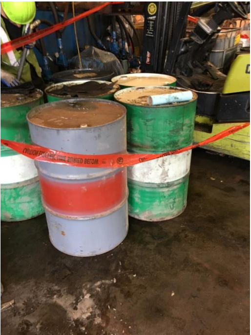
Improperly stored and labeled chemicals
