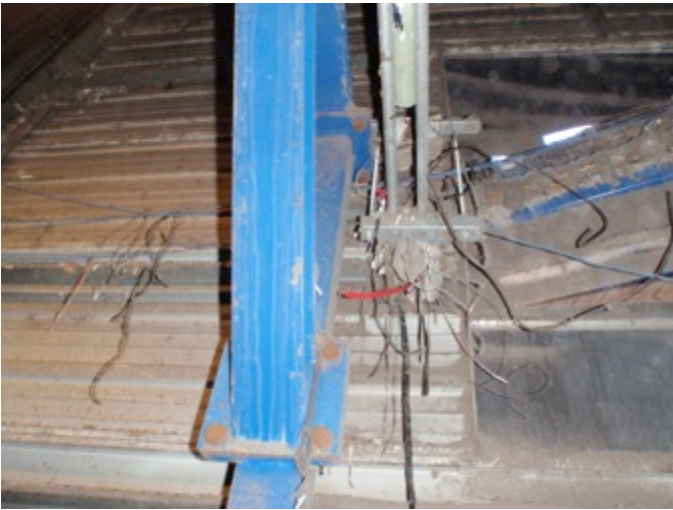
Top left: wiring under conveyer with debris over/under/on/around wire
