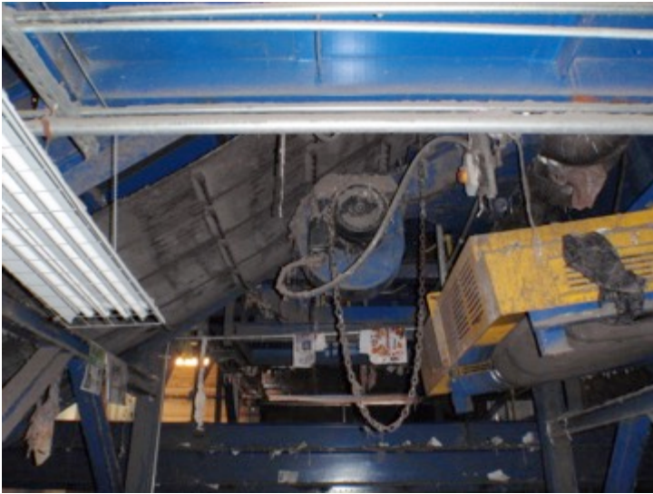
Top left: dust & debris atop electric motor
