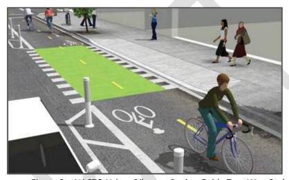
Figure 2 – NACTO Urban Bikeway Design Guide Two-Way Cycle Track Illustration
