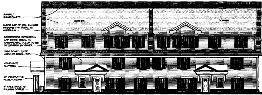
ALT. 'BI' FRONT ELEVATION-WEST (south building) PITCHED ROOF SCALE: 1/8" = 1'-0"
